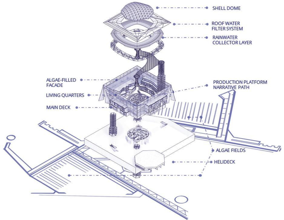
Fig. 7 - Exploded Axonometric (Kaan Çetin).
