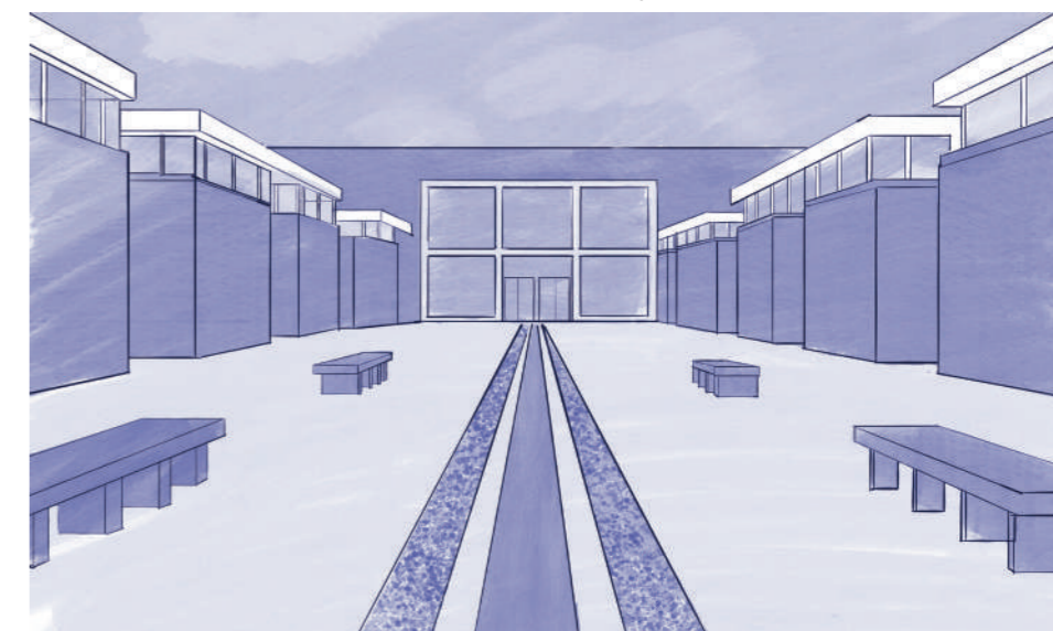
Fig.3 - Running water directing towards the entrance with a gravel strip either side to guide VI people alongside the water rather than into it.
