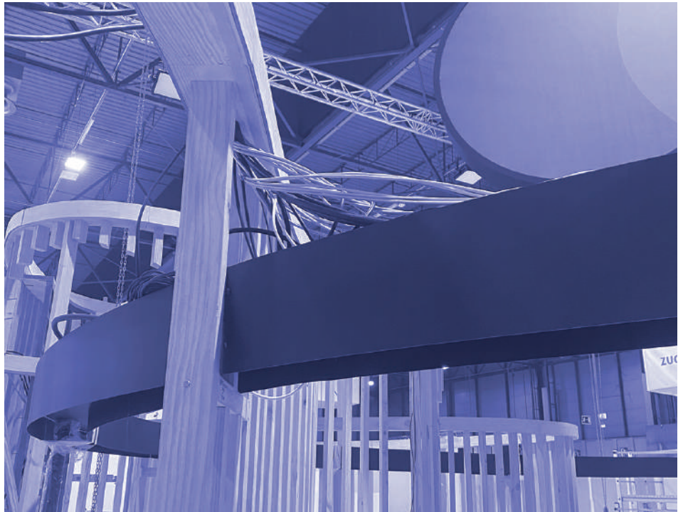
Fig. 9 - The black central ring as wiring distributor.
