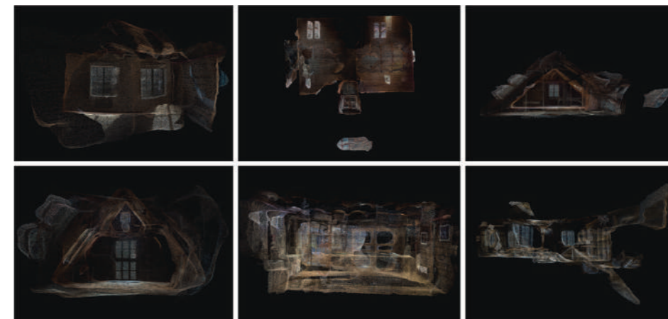
Fig.5 - Point cloud from 3d scan of a historic site in Bryggen, Bergen (Norway).
