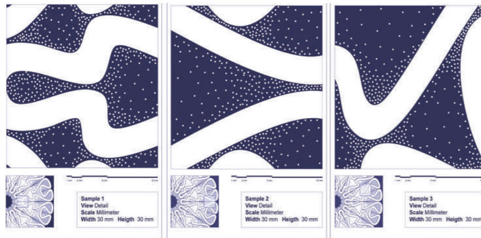
Fig.4 – Thirty-millimeter square samples showing the functionally graded material and the moisture fields.
